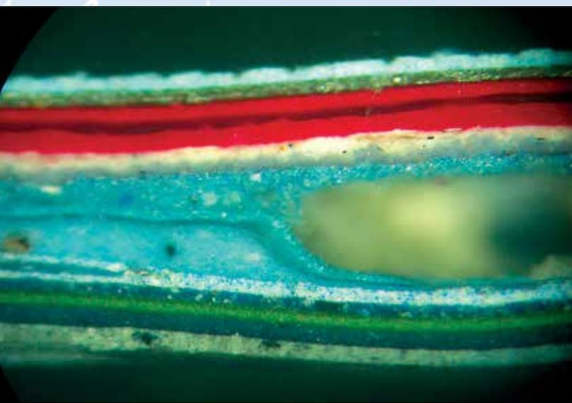
A microscopic cross section of paint layers on a car that was often repainted.
