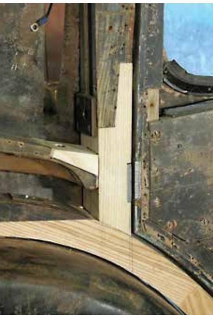
A restorer at Autoservice René Große planishes a large panel using a pneumatic hammer; the wooden frame of a Hispano-Suiza is given a partial restoration; this model for a Bugatti fender was made by laser-scanning an intact fender, flipping the image, and using a water-jet cutter.
