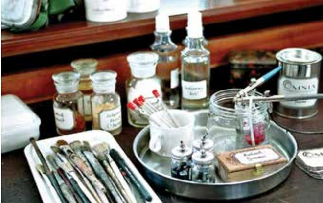
Airbrush equipment is used to retouch paints. Right: Gundula Tutt injects a special formula to consolidate the chipping original nitro paint layers on a Voisin C 11.
