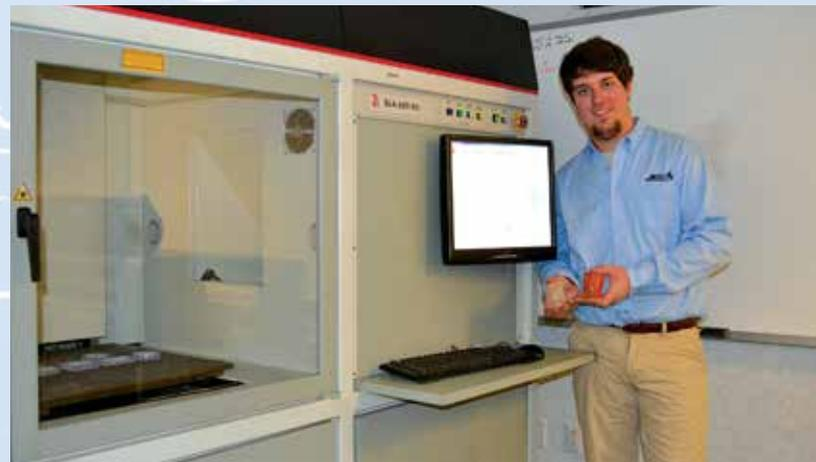
Pat Knapp holds the rear directional lens for a 1957 Ferrari 250 Tour de France Berlinetta. CAD technology was first used to create a template from the original broken pieces and then the design was perfected using SLA (sterolithography) rapid-prototyping technology.
